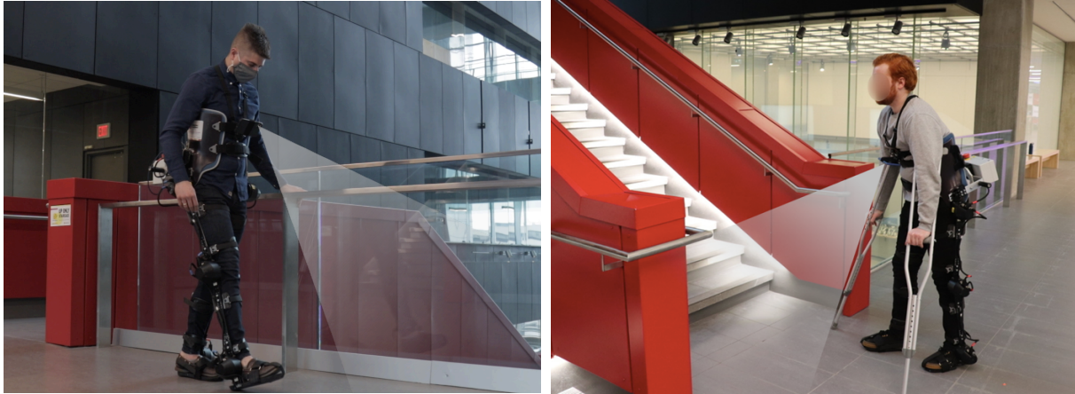
Figure 2.3. Examples of walking with a robotic lower-limb exoskeleton with computer vision-based environment sensing superimposed.
