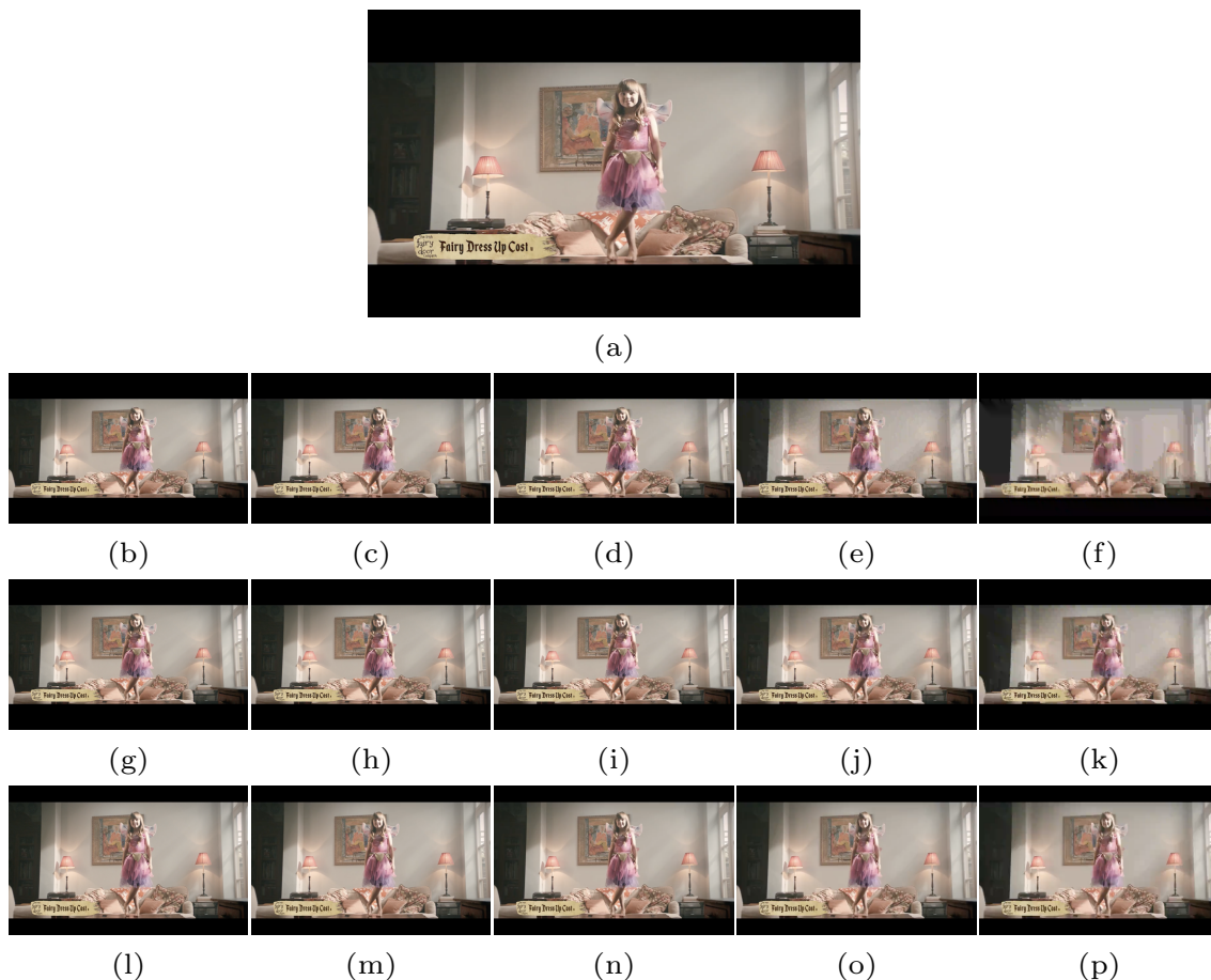
Figure 7.2: Sample frames of H.264 encoded videos in the Waterloo Streaming Video database. All images are cropped for neat presentation. (a) Source reference video frame. (b)-(f) 1920 \times 1080 at 8,000 kbps, 4,000 kbps, 1,000 kbps, 500 kbps, and 100 kbps. (g)-(k) 1280 \times 720 at 8,000 kbps, 4,000 kbps, 1,000 kbps, 500 kbps, and 100 kbps. (l)-(p) 740 \times 480 at 8,000 kbps, 4,000 kbps, 1,000 kbps, 500 kbps, and 100 kbps.
