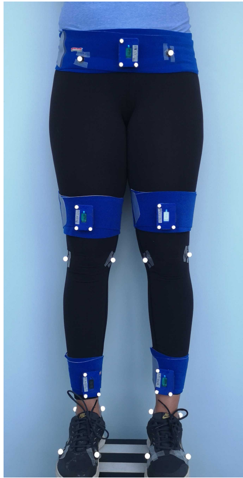
Figure 5.7 The placement of torso, knee, and ankle IMUs for the squat exercise is shown here, as well as the locations of the motion capture markers for ground truth joint angle trajectory estimation.
