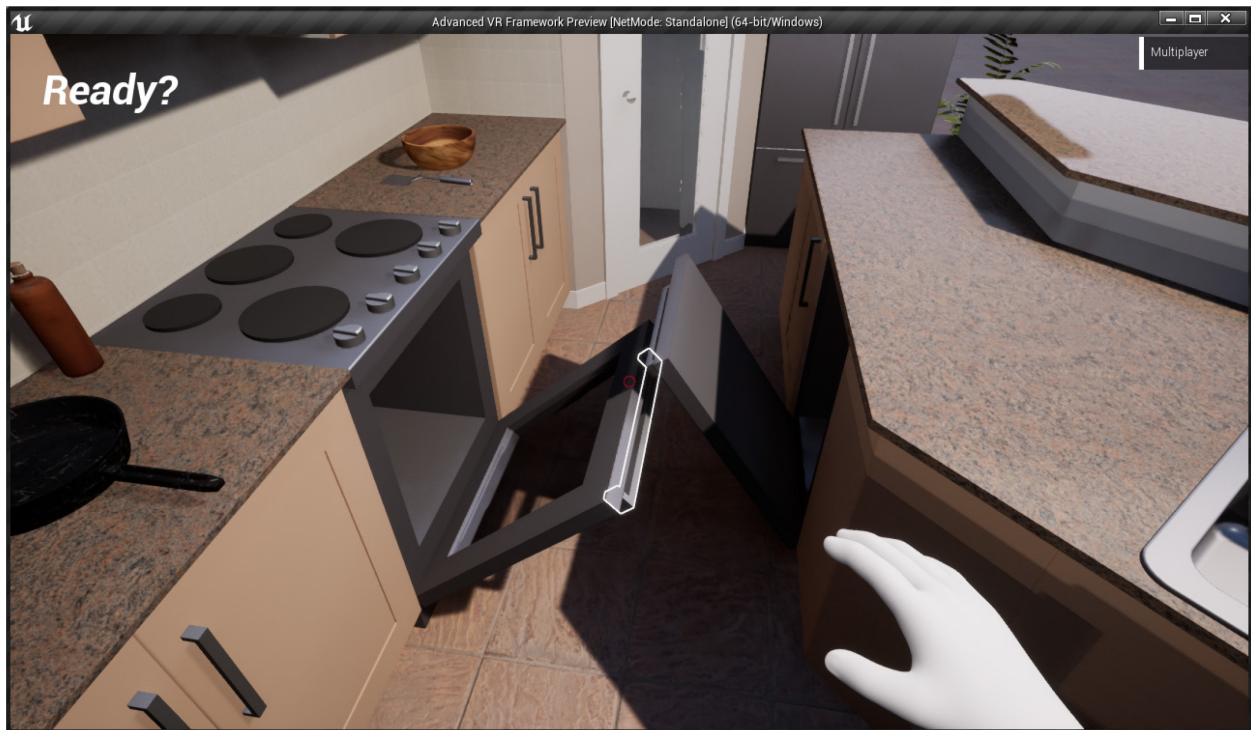
Figure 64. User finds that the doors to the oven and dishwasher clash during use. (Source: By Author)
