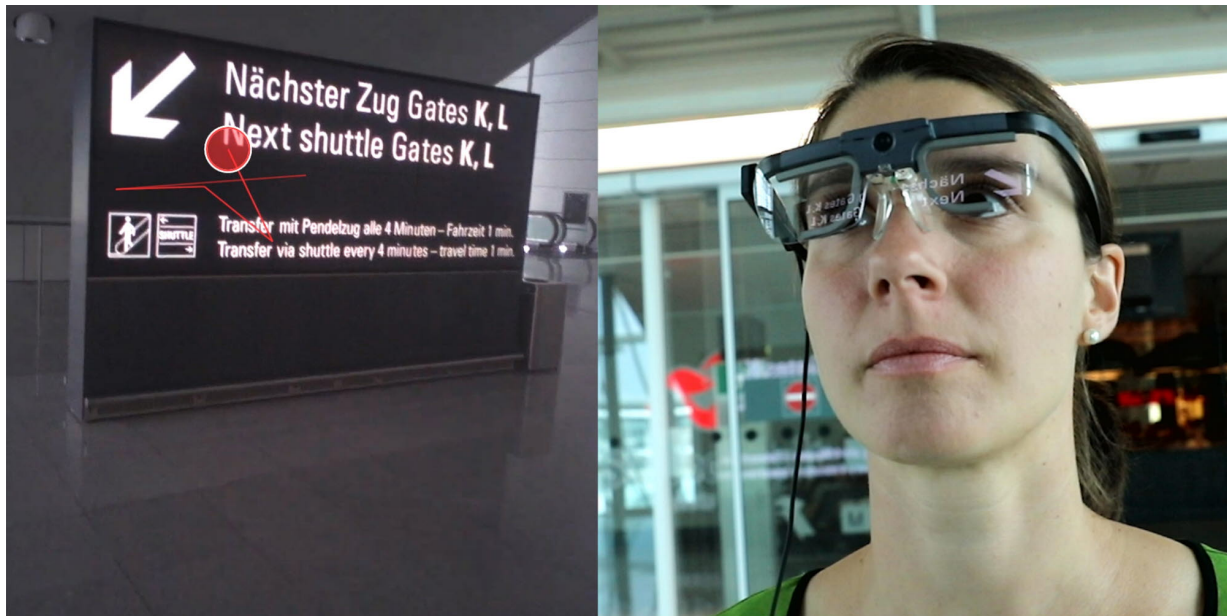
Figure 39. Woman wearing eye tracker glasses to identify what parts of Munich Airport she was looking at for wayfinding. (Source: Tobii Pro / Downloaded from https://www.tobiipro.com/applications/marketing-user-research/case-studies/munich-airport-study/ on January 2021)
