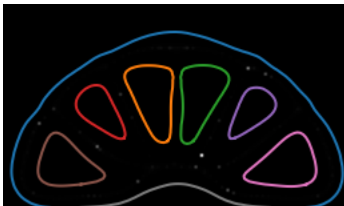
Figure 5.19: Diagram showing features increasing in thickness as the overhanging angle increases
