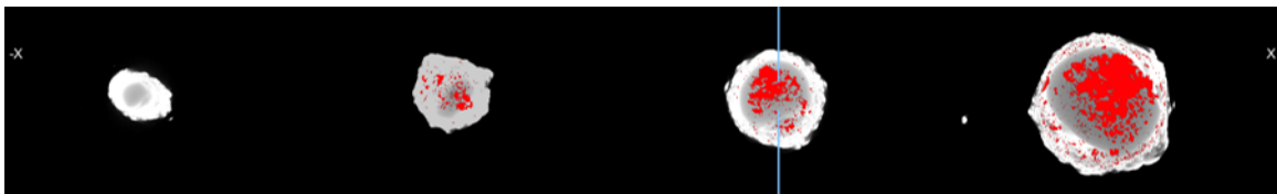
Figure 3.13: Top view of the porosity distribution for solid struts of different sizes (30° orientation). Pores are in red
