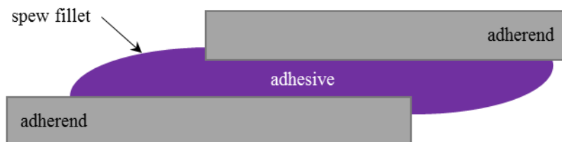
Figure 2.20: Side view of single-lap shear test specimen with spew fillet at the leading edges of the overlap
