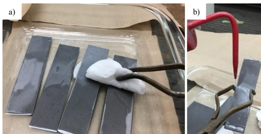
Figure 3.23: a) Swipe the adherend using a cotton pad to remove visible debris b) Wash off the remaining lint or fabric from the cotton pads
