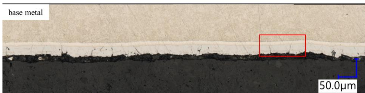
c) Boron steel in-die quenched at 700°C
