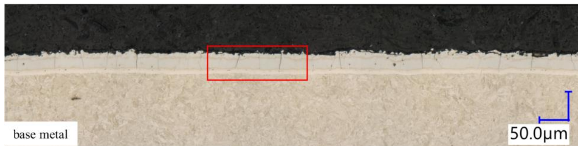
b) Boron steel in-die quenched at 400°C
