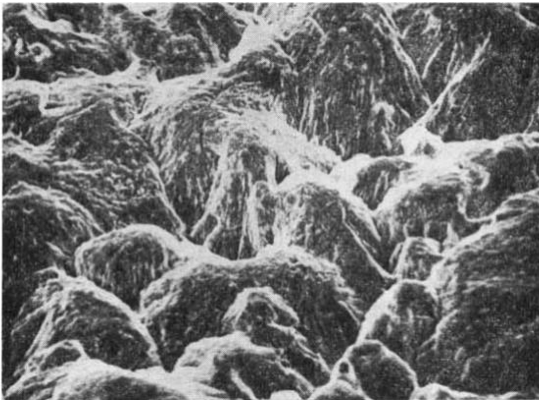
Figure 2.29: Sulphuric acid (H 2 SO 4 )/oxalic acid etched martensitic FV-520B stainless steel (x 1000) (Allen and Alsalam, 1976)
