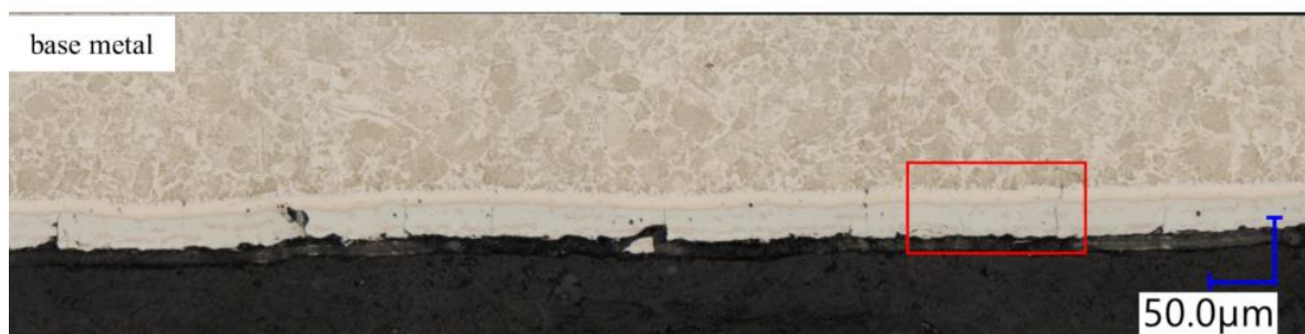
Figure 4.15: Microcracks in Al-Fe-Si coated boron steel in-die quenched at a) RT, b) 400°C, and c) 700°C
