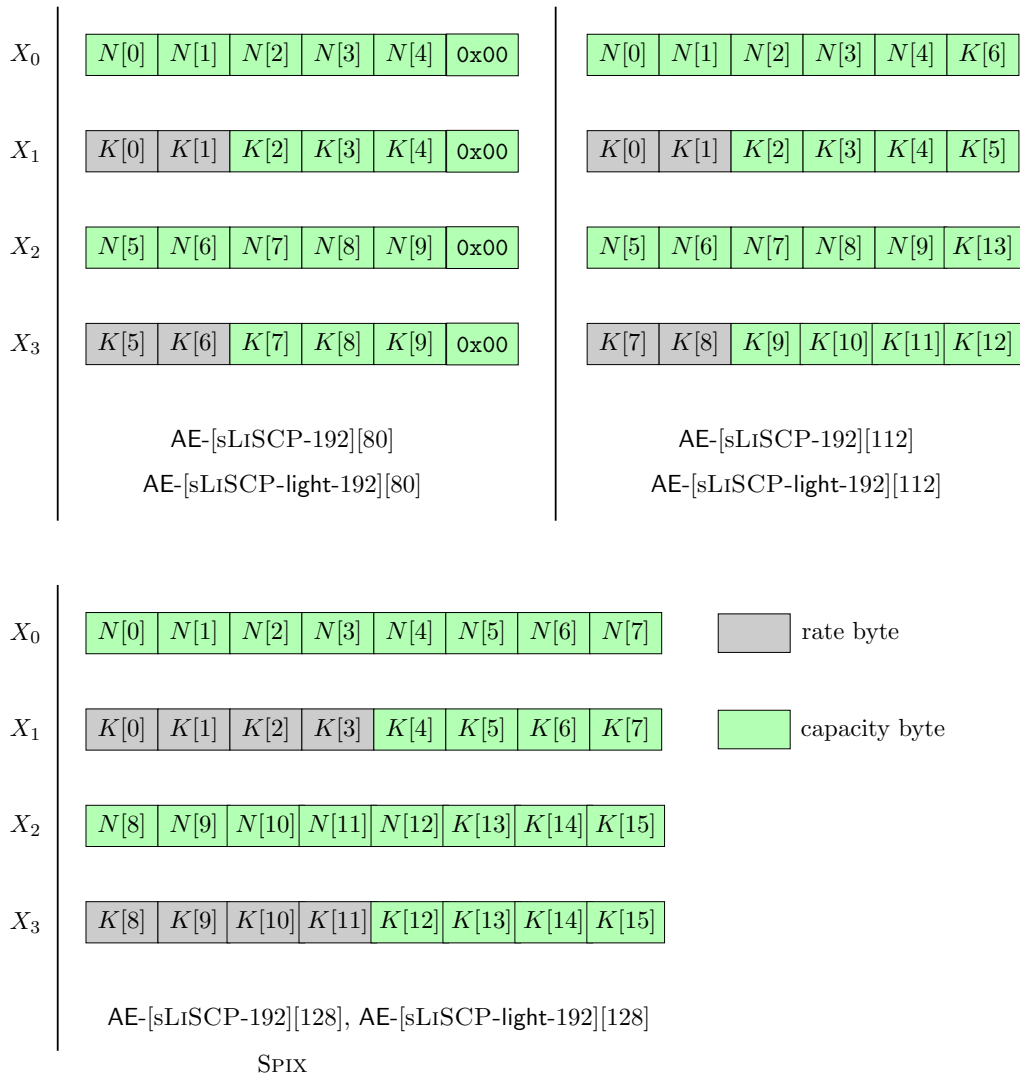
Figure 6.4: Visualization of load-AE(.) procedure of different AEAD instances
