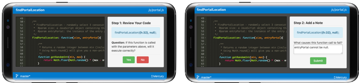
(a) Step 1 of Grounded Microtasks ask the user to assess the behavior of a function with a particular set of function parameters. (b) Step 2 of Grounded Microtasks allow the user to add a note alongside the function parameters that cause the function to fail.
