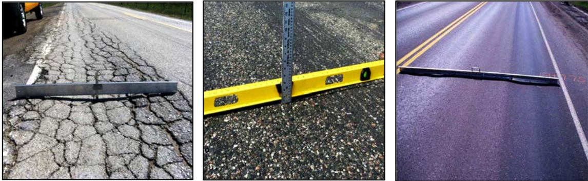
(a) Rutting on the pavement surface
