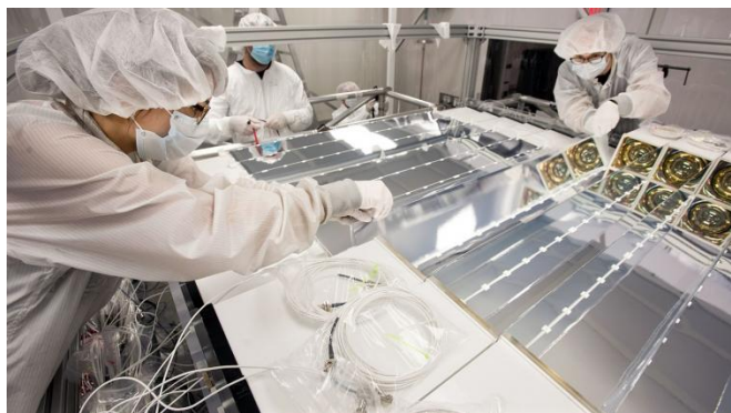
Figure 22: Detector assembly midway through the top row. A vertical reflector optical separator is inserted into the pinwheel arms (white tabs) and between housings. The white PMT housing bodies and clear front windows are visible on the near side while the far side shows the PMT faces and reflective cones. The top reflector optical separators were installed after all PMT housings and vertical reflectors of that row were installed.
