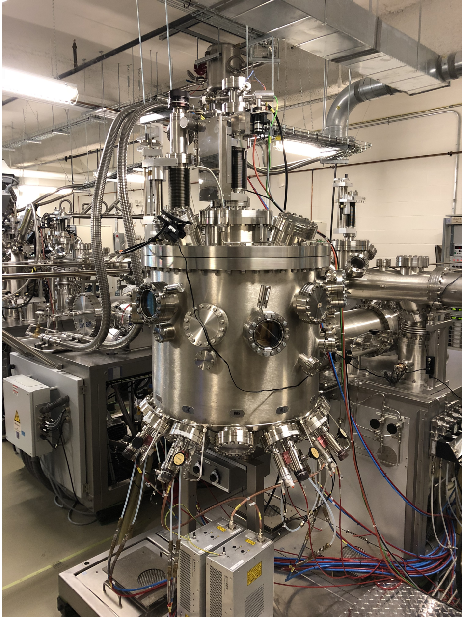
Figure 3.1: Omicron UHV sputtering system used to deposit Niobium films onto the sapphire wafers.
