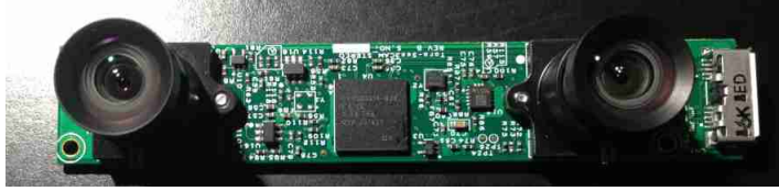
Figure 3.13: Tara stereo camera with built-in IMU.
