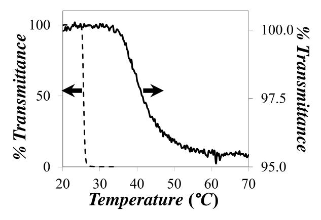
**Figure 6.** Plot of transmittance at 400 nm versus temperature for the PMEO<sub>2</sub>MA<sub>138</sub> homopolymer solution (- - - -) and the PEG<sub>113</sub>-b-PMEO<sub>2</sub>MA<sub>77</sub> copolymer solution (——).
