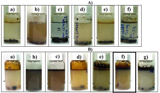
**Figure 8.** A) Extraction without toluene: a) pure water, b) 100 mM SDS, and 1 mg/mL aqueous solutions of c) PEG, d) PMEO<sub>2</sub>MA, e) PEG<sub>113</sub>-b-PMEO<sub>2</sub>MA<sub>77</sub>, and f) PNIPAM. B) Extraction with 60 mg toluene: a) pure water, b) 100 mM SDS, c) 200 mM SDS, and 1
