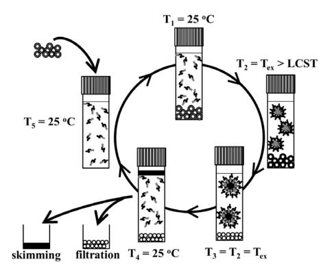
**Figure 1.** Proposed process for oil extraction from oil sands by using the thermo-responsive block copolymer PEG-*b*-PMEO<sub>2</sub>MA.
