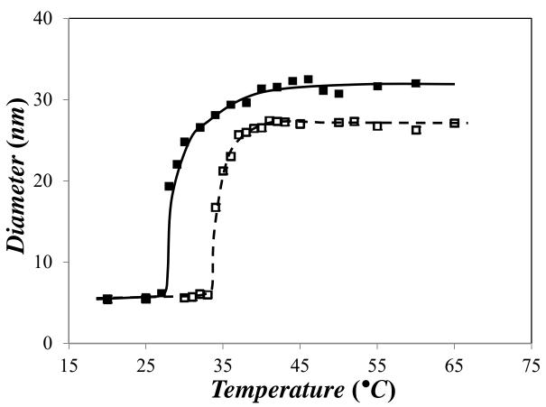
**Figure 10.** Plot of  $D_h$  as a function of temperature for a 5 mg/mL PEG<sub>113</sub>-b-PMEO<sub>2</sub>MA<sub>80</sub> aqueous solution with ( $\blacksquare$ ) or without ( $\square$ ) toluene. Lines are used to guide the eye.
