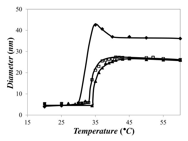
**Figure 7.** Plot of the hydrodynamic diameter ( $d_h$ ) as a function of temperature for the block copolymers PEG<sub>113</sub>-b-PMEO<sub>2</sub>MA<sub>64</sub> ( $\square$ ), PEG<sub>113</sub>-b-PMEO<sub>2</sub>MA<sub>77</sub> ( $\spadesuit$ ), and PEG<sub>113</sub>-b-PMEO<sub>2</sub>MA<sub>80</sub> ( $\blacktriangle$ ) in water. Polymer concentrations equal 5 mg/mL. Lines are used to guide the eye.
