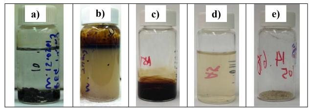
**Figure 2.** a) Before extraction: Mixture of oil sand particles at the bottom, 15 mL of 1 mg/mL PEG<sub>113</sub>-*b*-PMEO<sub>2</sub>MA<sub>77</sub> aqueous solution, and 60 mg of toluene on top of the solution. After 24 hrs extraction at T = 45 °C: b) Mixture with the extracted oil at the top of the aqueous solution; c) Oil recovered from the extraction; d) PEG<sub>113</sub>-*b*-PMEO<sub>2</sub>MA<sub>77</sub> aqueous solution; e) Pristine sand particles.
