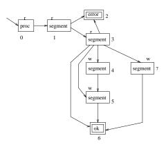
Figure A.11: The finite state machine of **brk**
