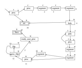
Figure A.7: The finite state machine of **fork**
