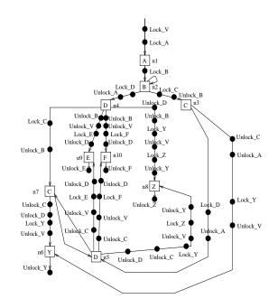
Figure 3.9: Transaction type with locking/unlocking steps (the solid cycles) inserted.
