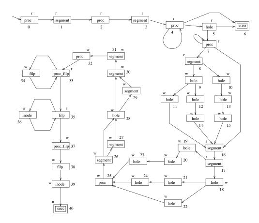
Figure A.10: The finite state machine of  $\mathbf{exec}$
