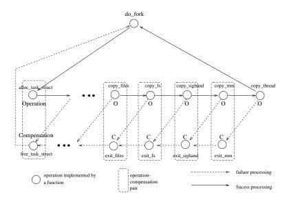
Figure A.1: The control flow of **fork**
