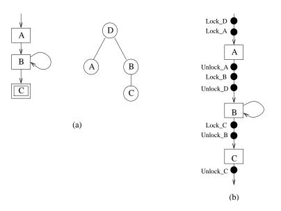
Figure 3.4: Adding lock states to a transaction type: (a) original transaction type and its local lock tree; (b) expanded transaction type.
