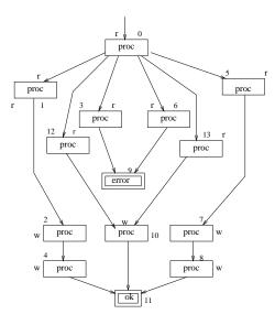
Figure A.9: The finite state machine of **waitpid**
