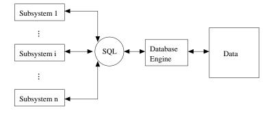
Figure 1.2: Database repository architecture
