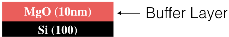
Figure 4-4 Deposit 10nm MgO (100) as the Buffer layer after heating the holder for 1 hour under 300°C
