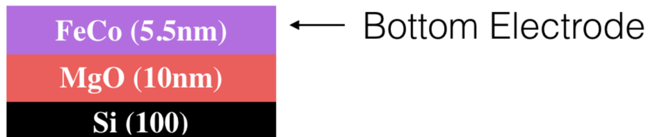
Figure 4-5 Deposit 5.5nm FeCo (100) through the bottom electrode shadow mask after cooling down the system from 300°C for 2 hours (approximately reaching 100°C)
