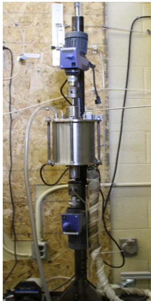
Figure 5-2: Picture of the double stirred tank reactor
