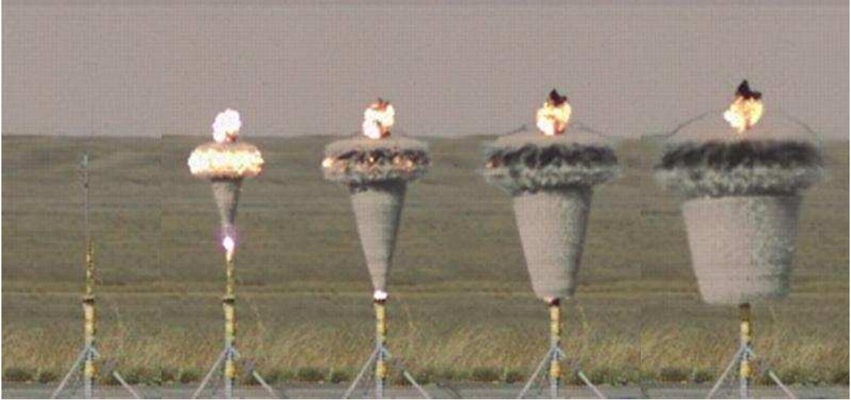
Figure 1.6: Cylindrical heterogeneous detonation and inert particle dispersal of 114\ \mu\text{m} aluminum particles in a 19 mm diameter tube from Frost et al. [74, 76]. Five instances in time shown with 114\ \mu\text{s} between frames. High-speed photographs from Defence R&D Canada – Suffield, courtesy of Dr. David Frost.
