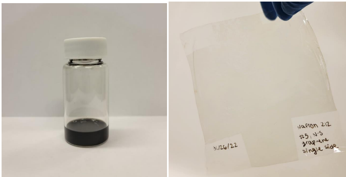
Figure 12. (Left) G-DMF ink for deposition prepared at an initial concentration of 0.42 mg/mL. (Right) Nafion membrane (approximately 7.5 cm x 8 cm) coated with a single monolayer of graphene. Reproduced with permission from [1].
