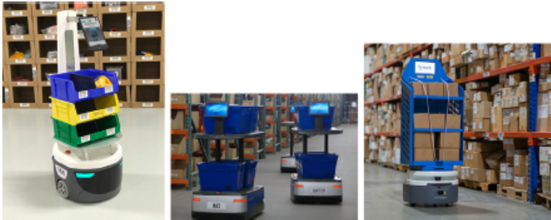
Figure 1.1: Example of autonomous picking cart from Locus Robotics, 6 River Systems, Fetch Robotics (Xie et al., 2022).
