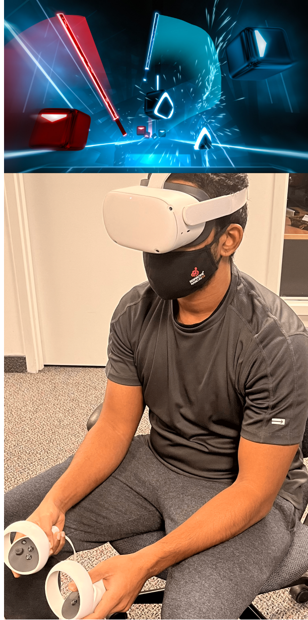
Figure 4.5: Oculus demo which provides vibrotactile haptic feedback from its hand-held controllers when the user strikes a block in a VR game called Beat Saber
