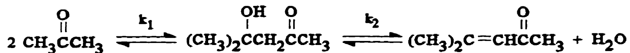
Figure 2.1-2: The aldol condensation of acetone to diacetone alcohol, followed by dehydration to mesityl oxide.
