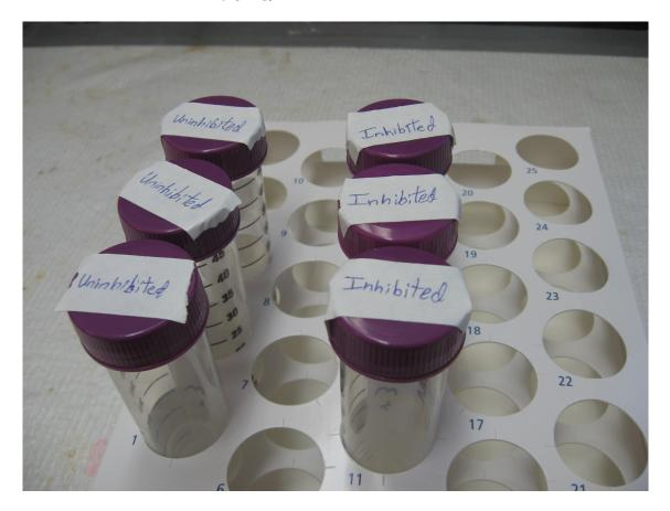
Figure 5.1: The batch test used in this study consists of inhibited and uninhibited batches being run in parallel.
