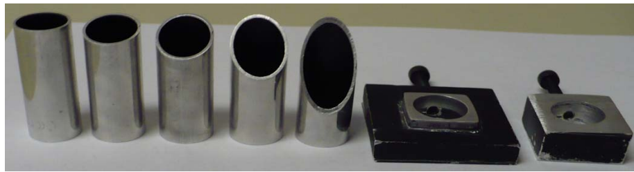
Figure 3.7: A Set of Fixed Sample Holders, Transmission and Reflection Adapters
